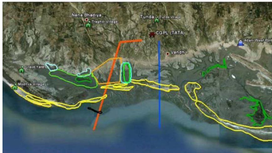
Fig. 4: Map showing intake and outfall channels, different habitats mapped. (Blue line: intake channel; Orange line: outfall channel; Dark green area: dense mangrove patch; Light green area: sparse mangrove cover; Light blue area: Potential sites for mangrove plantation; Yellow area: sand dunes; Dark yellow area: salt pans; Black area: rocky beds)
